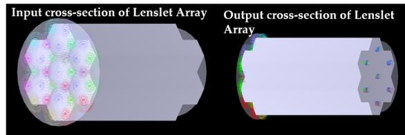
Figure 5: Optical layout of center and 1st ring of lenslets with 6 arcsec FoV
