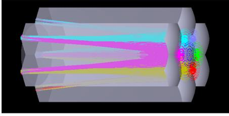
(a) Optical layout of center FoV (2 arcsec distribution) with center and 1st ring of lenslets
