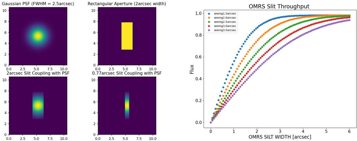
(a) PSF coupling with Slit (b) OMRS Slit Throughput In cassegrain Mode
