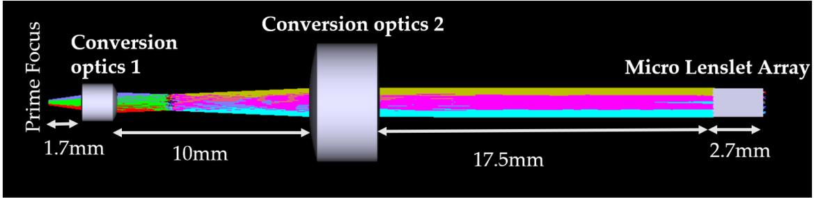
Figure 3: OMRS optical design for Prime mode with lenslet
