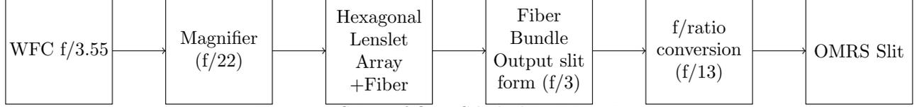
Figure 2: Setup of OMRS linked in Prime Focus
