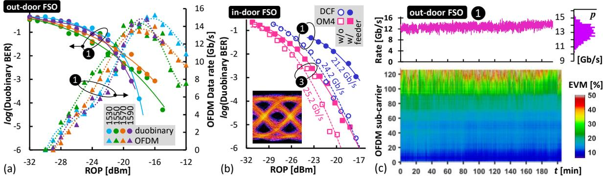
Fig. 4. Transmission performance for (a) out-door and (b) in-door FSO links. (c) Longer-term OFDM performance over out-door FSO link.
