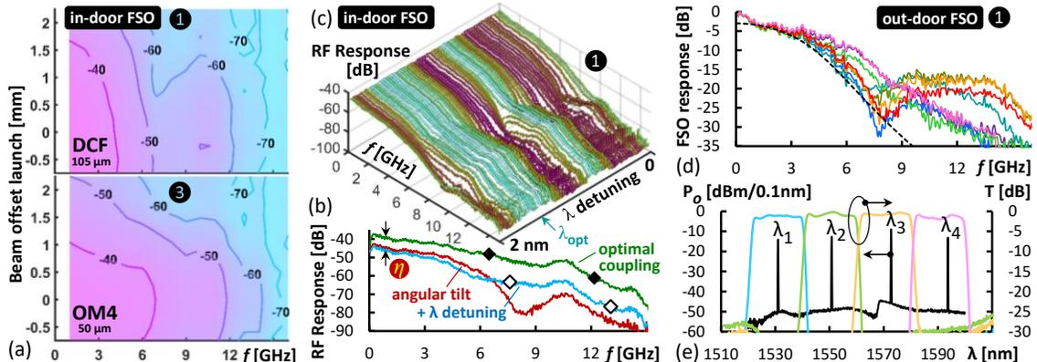
Fig. 3. In-door FSO bandwidth for (a) beam offset and (b) tilt, while (c) detuning  $\lambda$ . (d) Out-door FSO bandwidth. (e) Launched FSO channels.
