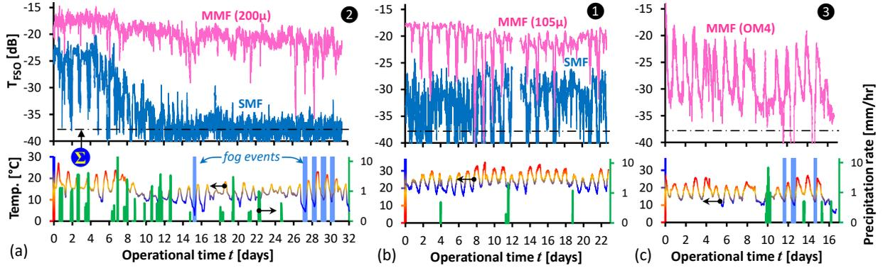
Fig. 2. FSO channel transmission for (a) DCF with 200- $\mu\text{m}$  MMF and (b) 105- $\mu\text{m}$  MMF used as receiving fiber. (c) Comparison to OM4 fiber.
