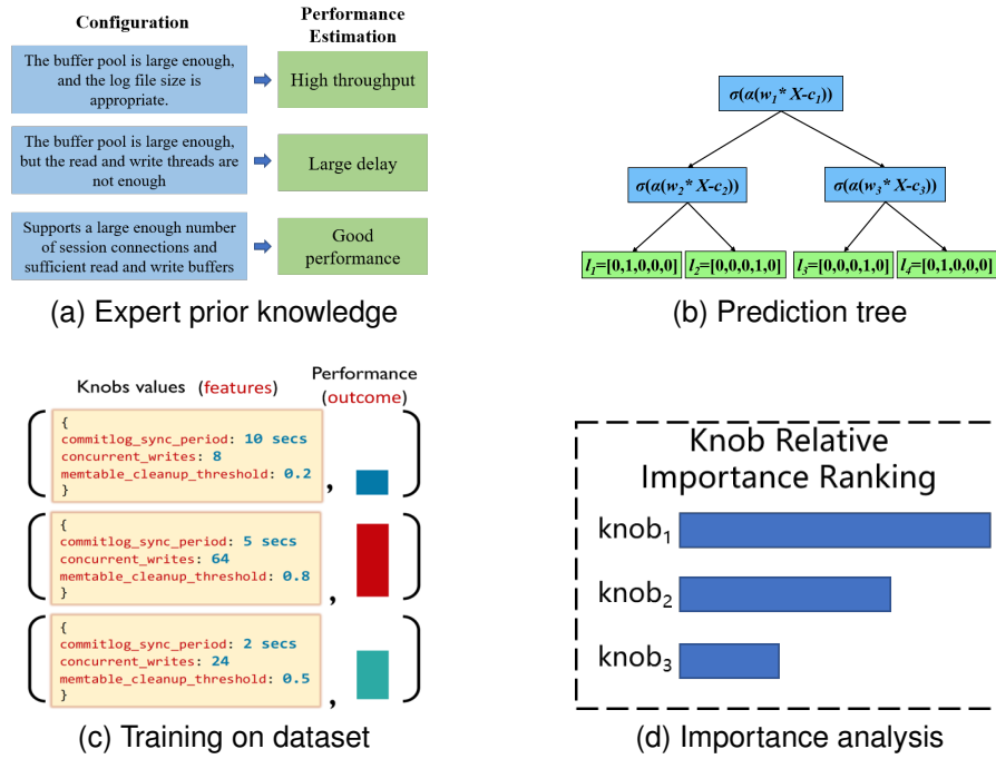
Fig. 2. The workflow of parameter selection. (a) Gathering expert knowledge; (b) Transforming this knowledge into a prediction tree; (c) Constructing a dataset and training the prediction model; (d) Analyzing parameter importance using Shapley values.
