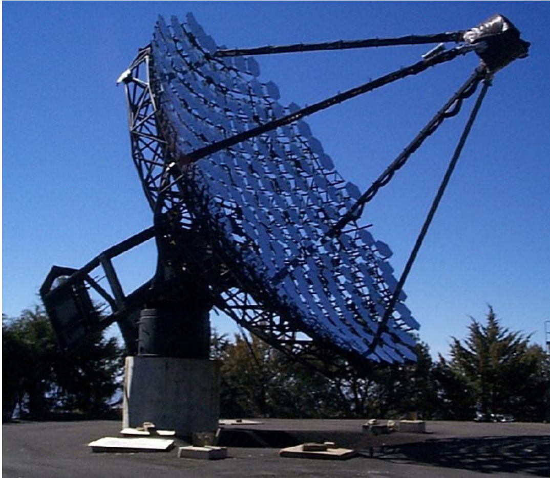
Fig. 2 Photo of the 10 m diameter pioneering Whipple IACT on mount Hopkins in Arizona
