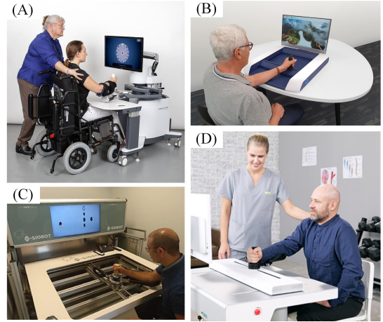
Fig. 1. End-effector rehabilitation devices. (A) InMotion [3] arm rehabilitation device, commercialized based on the multi-link MIT MANUS [4] design. (B) H-MAN [5] arm rehabilitation device, utilizing an H-shaped differential pulley and belt mechanism. (C) Physiobot arm rehabilitation device using a backdrivable linear actuated mechanism [6]. (D) ArmMotus M2 Gen [7] rehabilitation device utilizing a backdrivable linear actuated mechanism.
