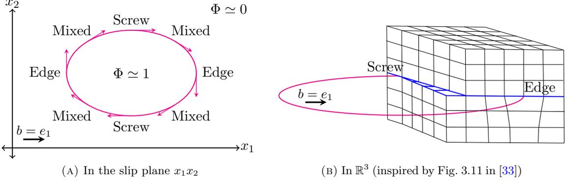
FIGURE 3. Dislocation types in a slip loop dislocation with fixed Burgers' vector
