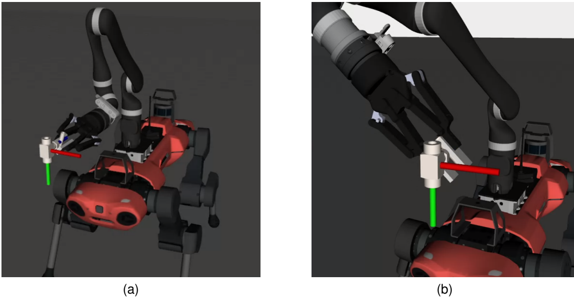
Fig. 5. Twisting a needle valve using the (5a) low-torque and (5b) high-torque strategies. The adaptive behavior can reactively select between these strategies.
