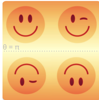
Figure 1. Illustration of the doubling step in the DFS method. The upper half shows a spherical map calculated on a rectangular grid and is mirrored along the \theta = \pi axis. The mirrored image is split in half across the \phi -direction in the center, and swapped. The result is a function on the torus, with a 2D ordinary Fourier series having the exact same band-limit as the spherical harmonic series of the original map defined on the sphere. This allows the use of efficient nonuniform Fast Fourier Transform for accurate interpolation.
