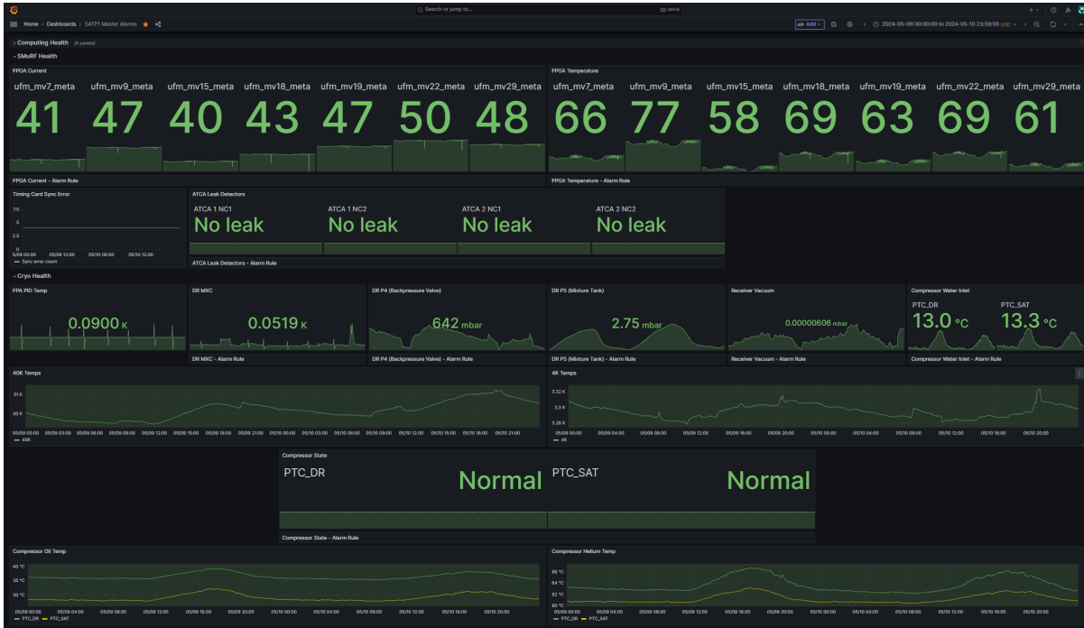
Figure 3: An example Grafana dashboard used to monitor metrics for one of the SATs. In this case, we show the health of the SMuRF system and the cryogenics system. This dashboard has a combination of different display types: time-series plots of temperatures, some with multiple sensors shown in the same plot, as well as ‘single-stat’ panels, which give the most recent value (for this case, the FPGA currents/temperatures and DR temperatures/pressures). Also shown are the single-stat states for binary flags from systems (in this case, that no leak is present in the system). Here, panels show green for normal operations. When thresholds are exceeded and alarms are triggered, the panels show red. Panels are grouped by the alarm groups described in Section 2.
