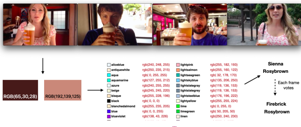
Fig. 8. Process of dominant colour detection based on one frame of the example video
