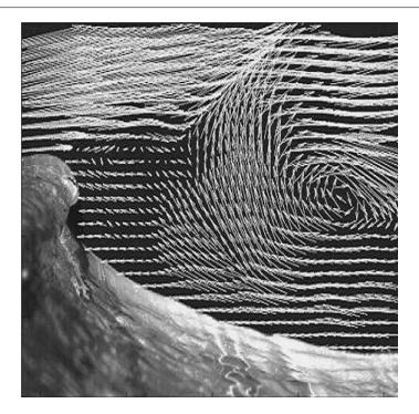
**Figure 6.** Jeffreys' mechanism - Airflow separation observed by "Particle Image Velocimetry" over a breaking wave [41]. The air pressure on the windward face of the wave is larger than the leeward face, which is the origin of continuous energy transfer from wind to wave.
