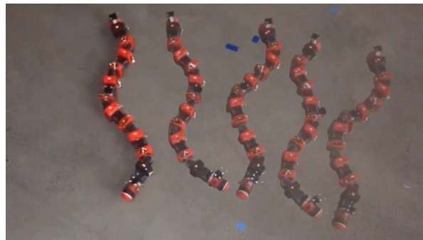
Fig. 1. Illustrates COBRA platform while performing sidewinding over flat ground.
