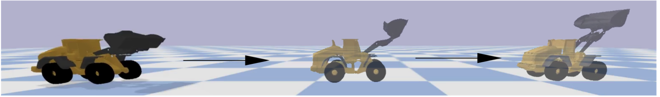
Fig. 2. The simulated setup where the agent should learn how to drive forward while lifting the bucket.
