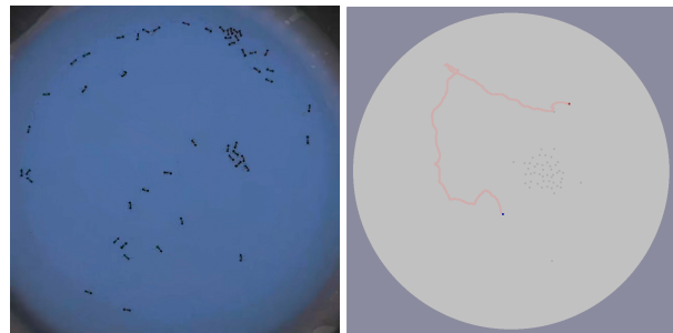
Figure 1: Left: Top-down video recordings, cropped and scaled to 1280x1280 resolution. The ants are filmed from above in an evenly-lit 100 mm diameter arena. Individual ant positions are extracted from a 4 hour recording. Right: Our simulation environment using Pygame and Gymnasium to reproduce ant colony dynamics with an agent that can interface with a policy network.
