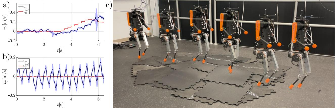
Fig. 10: The robot is able to traverse unknown unstructured terrain. Here it walked over a pile of rubber mats with a maximum height of 0.11 m. The reference velocity is shown in red, the filtered average velocity over half a step period is shown in black, with the shaded-area indicating the one standard deviation variation over half a step period. a) Velocity  $x$  tracking. b) Velocity  $y$  tracking. c) Snapshots of the rough terrain walking.
