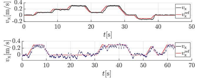
Fig. 8: Tracking a desired COM  $x$  velocity in simulation (top) and on hardware (bottom). The filtered state is calculated by using the moving average over one step period, 0.25 seconds. The blue bounds quantify the 1-standard deviation variation over one step period. On hardware, the reference signal was obtained via joystick control.
