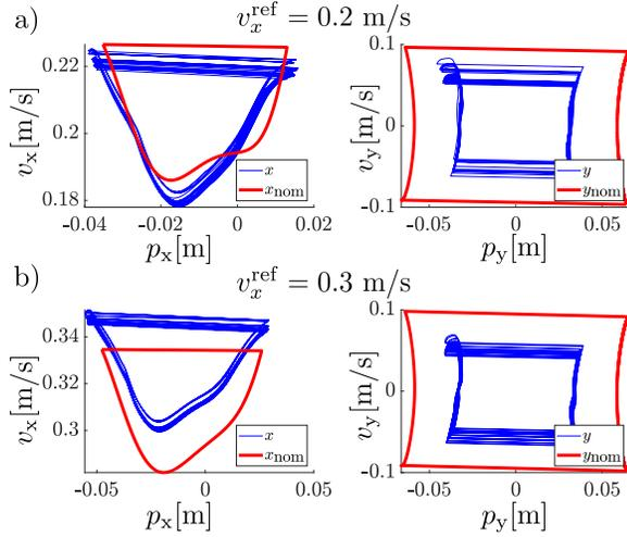
Fig. 7: Phase portraits of the simulated robot’s underactuated COM  $x$  and  $y$  states over several steps are shown together with the orbits from the nominal HZD gaits. a) phase portraits for reference velocity  $v_x^{\text{ref}} = 0.2$  m/s. b) phase portraits for reference velocity  $v_x^{\text{ref}} = 0.3$  m/s.
