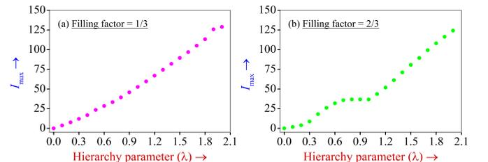
FIG. 6: Variation of the persistent current ( $I_{\max}$ ) as a function of the hierarchy parameter  $\lambda$  for a 4th generation SPG fractal structure with (a)  $\nu = 1/3$  and (b)  $\nu = 2/3$ .
