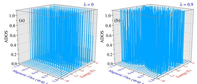
FIG. 4: Average density of states (ADOS) for a 3rd generation SPG fractal structure as a function of the energy and hierarchical magnetic flux. (a) is for  $\lambda = 0$  and (b) is for a non-zero value of  $\lambda = 0.9$ .
