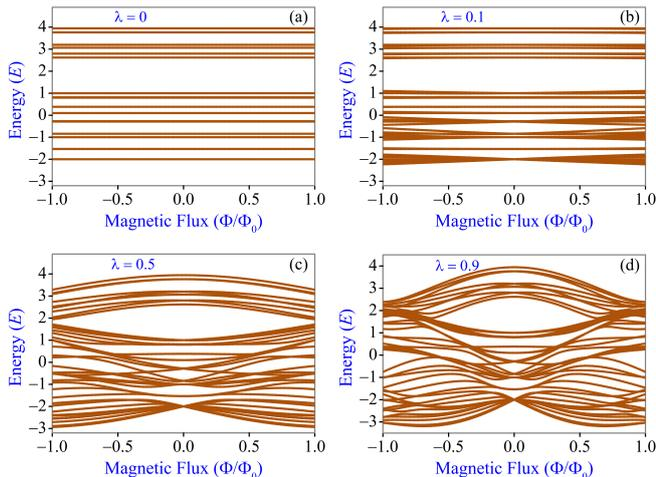
FIG. 2: Variation of the energy eigenvalue spectrum for a 3rd generation SPG lattice structure [with  $\mathcal{N}(3) = 42$ ] as a function of the hierarchical magnetic flux for different values of the hierarchy parameter, *viz.*, (a)  $\lambda = 0$ , (b)  $\lambda = 0.1$ , (c)  $\lambda = 0.5$ , and (d)  $\lambda = 0.9$ .
