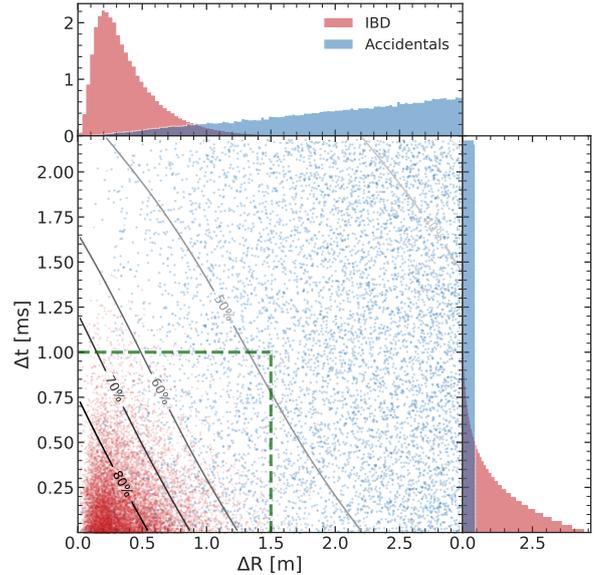
Figure 6: An example of a partial dependence plot for the following two features:  $\Delta R$ ,  $\Delta t$ . Solid lines represent different FCNN’s confidence levels that an event belongs to the IBD class. The green lines show the cuts selection criteria. Blue and red points show the events from the testing dataset.
