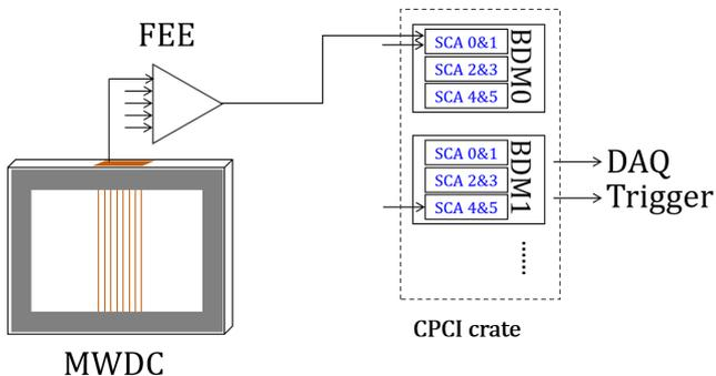
Fig. 4. (Color online) The schematic view of the electronics and the signal flow of the MWDC prototype.
