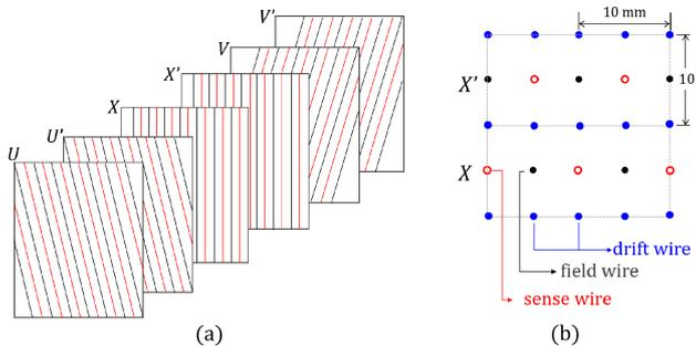
Fig. 3. (Color online) (a) The schematic view of the sense wire orientation, (b) The cross section view of the drift cells along X sense wires.
