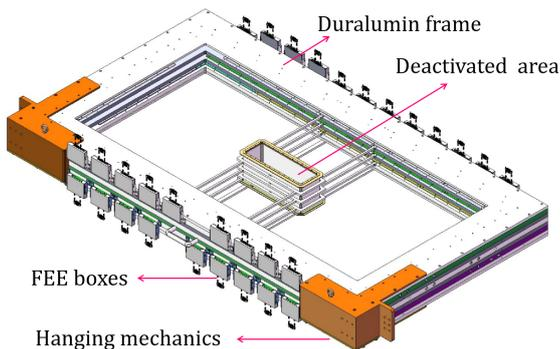
Fig. 10. (Color online) The mechanic structure of the MWDC. In the center is the inactive area, through which the unreacted beam particles pass through. The sensitive area of the detector is  $136 \text{ cm}(x) \times 63 \text{ cm}(y)$  and the deactivated area is  $30 \text{ cm}(x) \times 10 \text{ cm}(y)$ .
