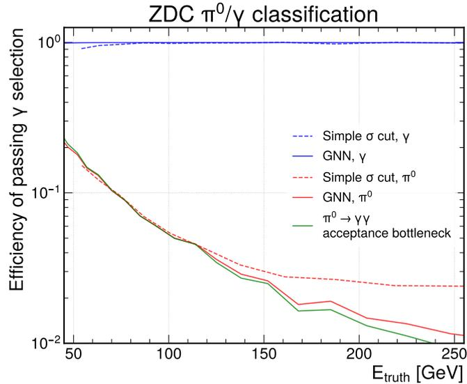
Figure 9: Efficiency of classifying  $\gamma$  (blue) and  $\pi^0$  (red) as  $\gamma$ . The  $\pi^0$  rejection efficiency has a bottleneck (green) at lower energies due to events with only one photon hitting the ZDC. The green curve quantifies the fraction of events where both decay photons hit the ZDC, and it hence shows the theoretical best classification performance.
