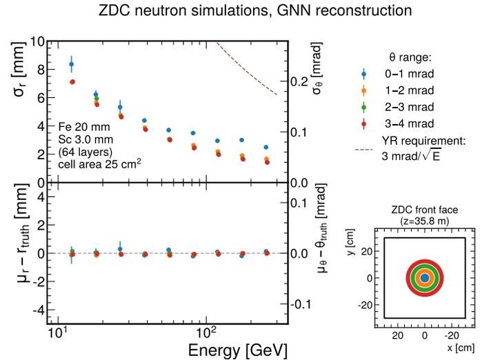
Figure 6: Top: same as Fig. 5, except in slices of  $\theta$  and only for the GNN method. Bottom: bias in position reconstruction for neutrons as a function of the generated energy. The colored regions in the inset provide a visualization of where these slices of  $\theta$  intersect the front face of the detector.
