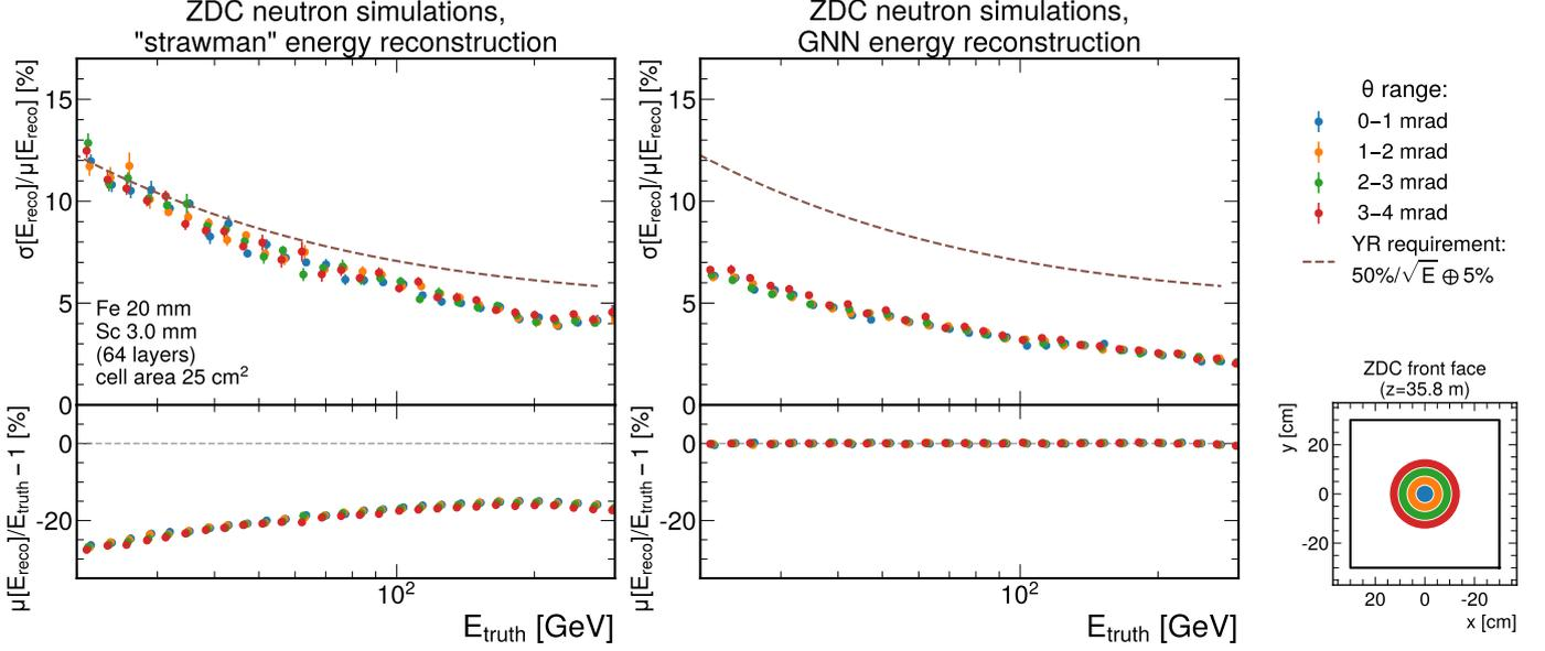
Figure 4: Energy resolution (top row) and scale (bottom row) obtained with the strawman (left) and GNN (right), at various ranges in  $\theta$ . The positions on the face of the detector corresponding to each color are visualized in the inset.
