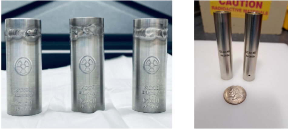
Figure 12: Left: Three custom-made AmLi sources used in LZ. The gold-ameridium-lithium matrix is encapsulated in nested tungsten and stainless steel capsules, which are designed to integrate with the CSD system and provide gamma-radiation suppression. The welds on the outer stainless-steel capsules are visible in the picture. Right: Two customized AmBe sources from Eckert & Ziegler designed for LZ. The stainless steel threaded capsules were designed to integrate in the CSD system and shield against low energy gammas from ^{241}\text{Am} decay.
