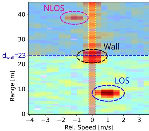
Fig. 5: Exemplary periodogram from the scenario presented in Sec. IV-A. The static return at  $d_{\text{wall}}$  is generated by the wall, and the joint LOS-NLOS returns from the moving target are highlighted. The NLOS region is highlighted in blue, discarded static bins in red.
