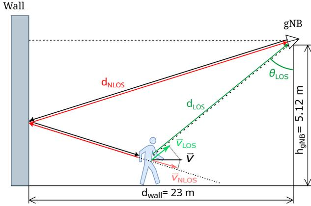
Fig. 4: Geometry of the measurement scenario. The target moves back and forth in a straight line between the wall and the gNB.
