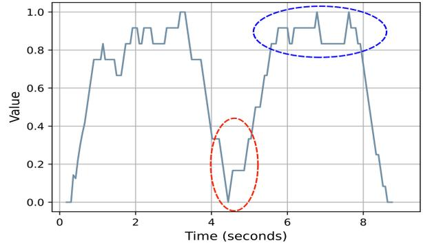
Fig. 6: Moving average of NLOS detections over a 0.5 s time window, using exponential threshold and clutter removal. Periodograms were generated using CSI matrices from  $K = 8$  frames.
