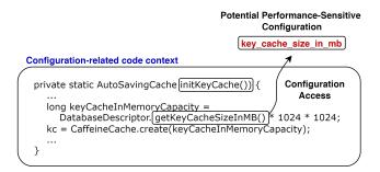
Figure 2: An example of performance-sensitive configuration.
