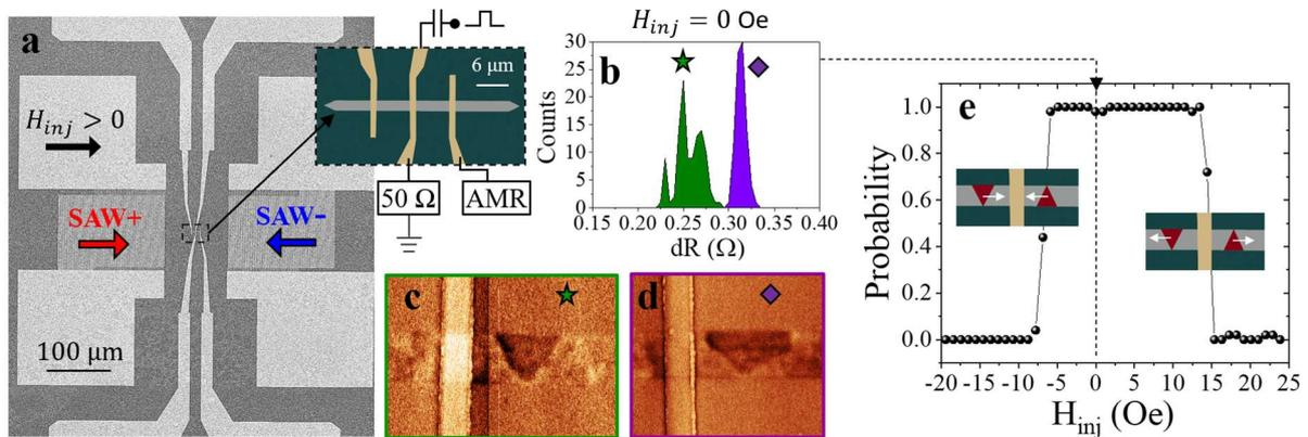
**Fig.1.** (a) SEM photograph of the device with the two IDTs that can deliver a SAW from left to right (SAW+) and from right to left (SAW-). In the inset, there is a colour-enhanced picture of the strip with the three contacts, where the middle one is used to nucleate the DWs and the lateral ones are used to measure the AMR of the DW. (b) Histogram of the
