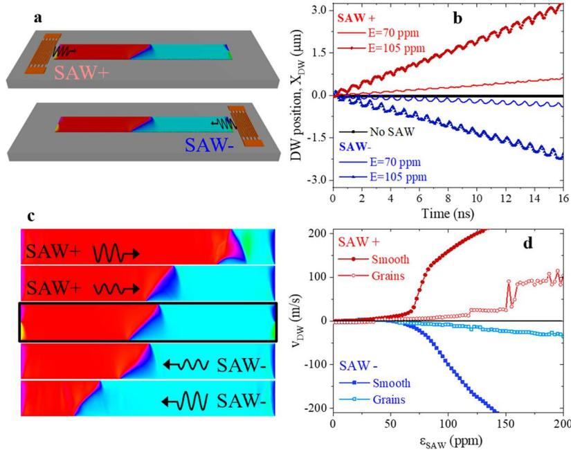
**Fig. 4.** (a) Set up with a single transversal DW nucleated in the middle of a FeCo strip where the SAW is delivered from both directions as indicated in the figure (b) Time evolution of the DW position along the nanostrip for several values of the SAW
