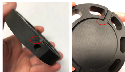
Figure 3: Flanges in Epoxy 82, fractures are visible near corners and sharp edges.
