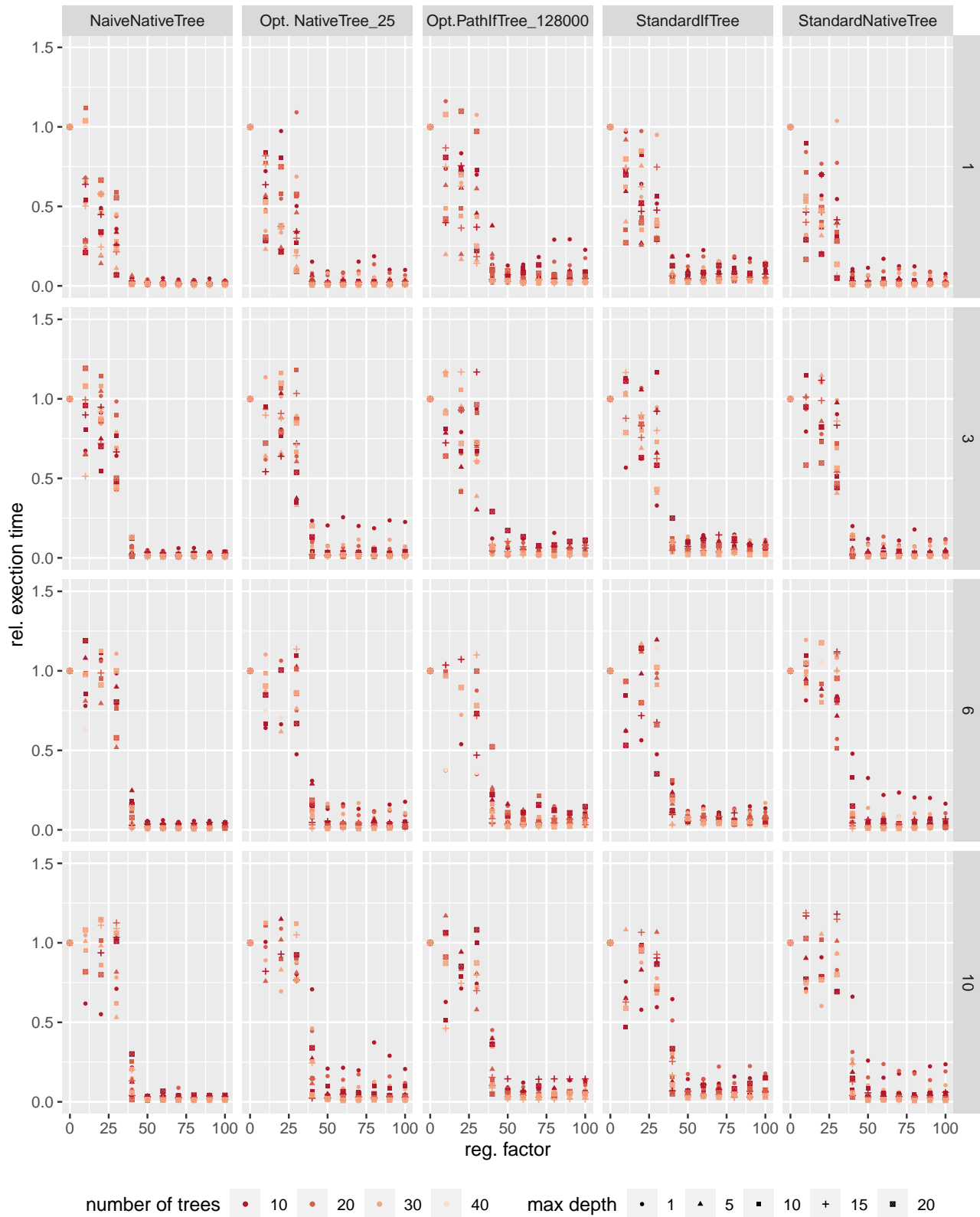
Figure 20. Relative execution time evaluation for synthetic data (red setting) and sample size=100 with varying sample size, max\_features , maximum depth (point shape) and number of trees (color).
