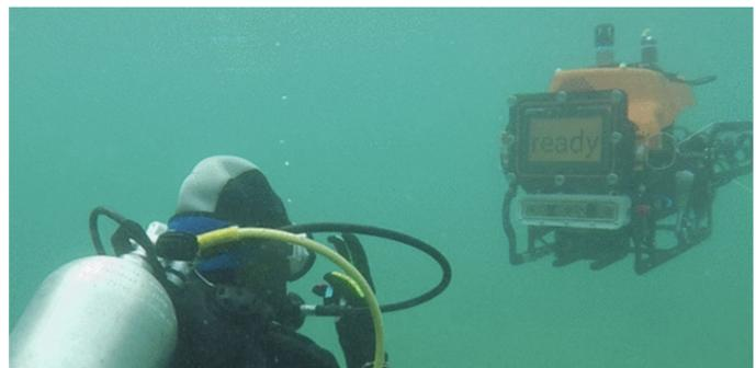
Fig. 1: Diver using hand gestures to communicate command to underwater vehicle [23].
