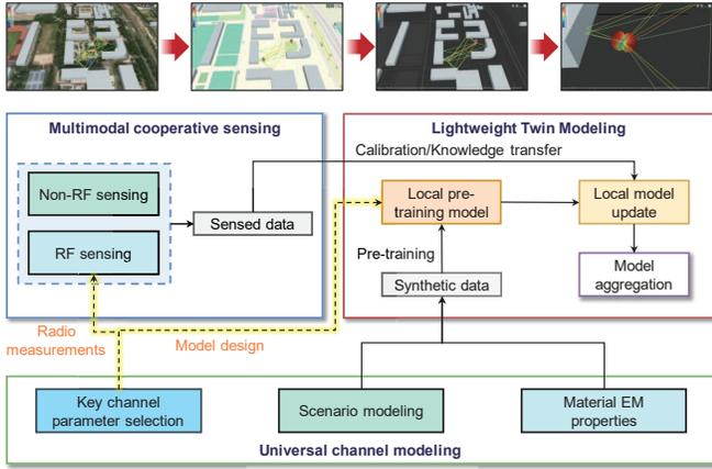
Fig. 2. The overall modularized CT architecture. The universal channel modeling module provides information about the sensing targets and prediction tasks of interest for the other two modules. The channel modeling module can generate synthetic data, which can be leveraged to pretrain the CT model in the lightweight twin module. Then, the CT model can be fine-tuned by feeding sensing measurements from the multimodal cooperative sensing module.
