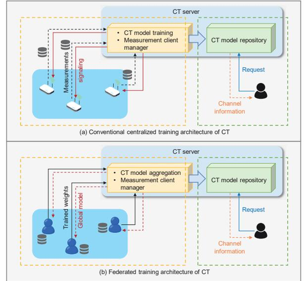
Fig. 3. Training architecture of CT: (a) Centralized learning-based CT model construction, where dedicated measurement anchors collect data and upload data to the CT server for training; and (b) FL-based CT model construction, where registered device clients use their local data to train the model and only upload trained parameters for model aggregation at the CT server.
