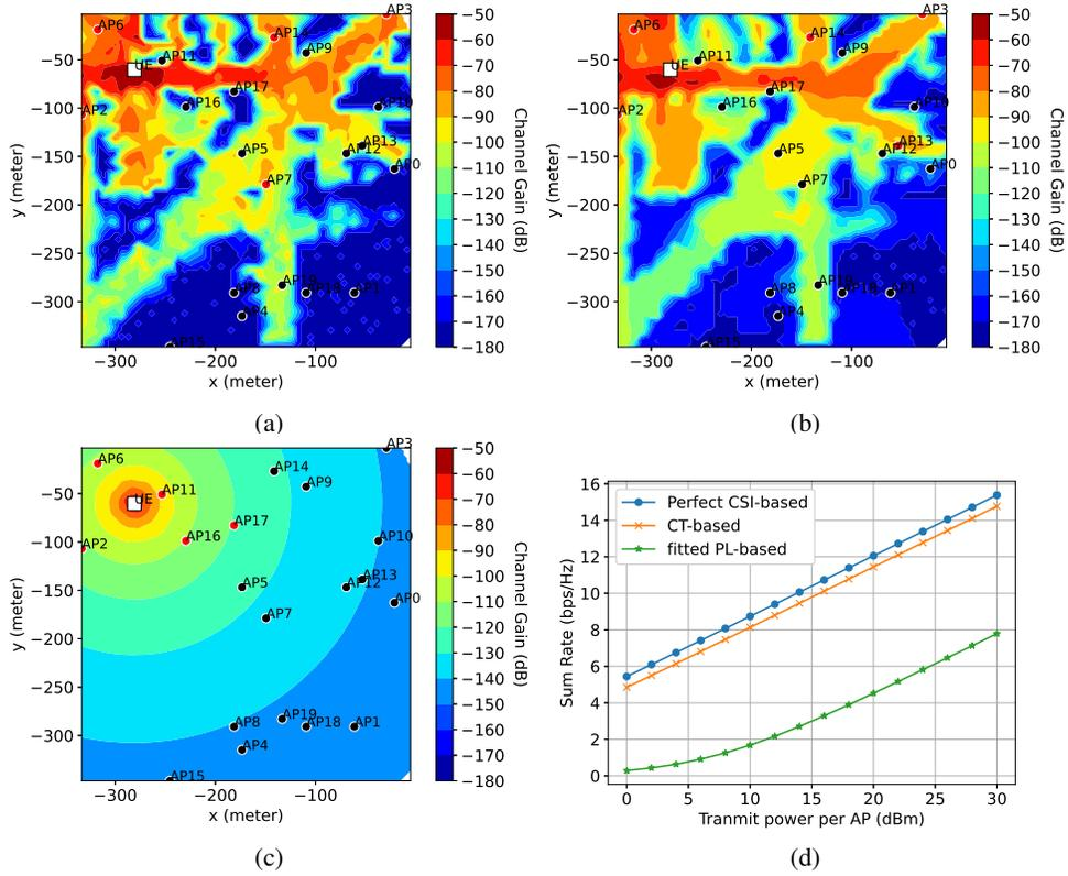
Fig. 4. User association results produced based on the true channel, the twin channel, and the fitted PL model: (a) True channel gain; (b) twin channel gain; (c) channel gain predicted by fitted PL model; and (d) the achievable sum rate with different schemes. Each UE selects five APs for communications, and the associated APs are indicated by red dots.
