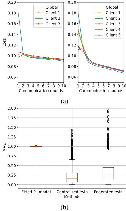
Fig. 5. Federated twin of the channel gains: (a) The validation loss versus communication rounds, where the total number of training samples is 10,000, and these samples are randomly divided into three or five UEs for FL; and (b) MAE comparison of channel gain prediction across different models.
