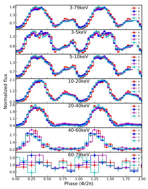
**Figure 3.** Energy-resolved pulse profiles of 4U 1538-522 in seven different energy bands (from top to bottom, 3-79 keV, 3-5 keV, 5-10 keV, 10-20 keV, 20-40 keV, 40-60 keV, and 60-79 keV). Different colors (red, blue, purple and cyan) represent 1-4 *NuSTAR* observations. For the sake of comparison, all pulse profiles were normalized to their mean values.
