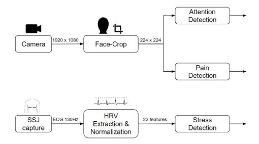
Fig. 5. Illustration of pipelines deployed for real-time prediction of attention, pain, and stress.
