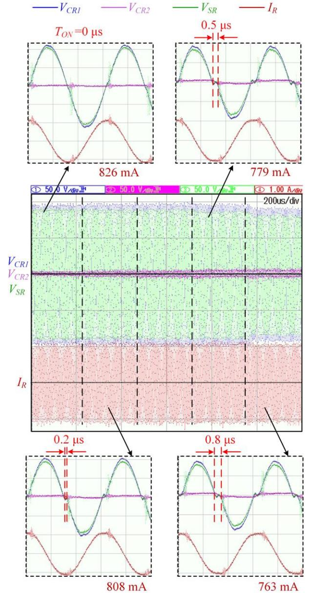
Fig. 15. Voltages and current of the hacking receiver under 161 kHz.
