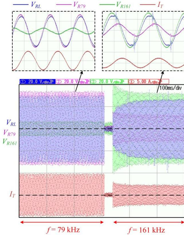
Fig. 16. Load voltages under different frequencies.
