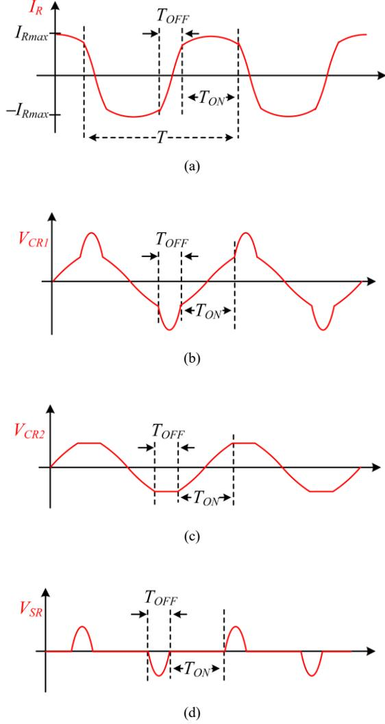
Fig. 3. Waveforms of system voltage and current with the time-division switched-capacitor array. (a) Receiver current. (b) The voltage of the capacitor  $C_{R1}$ . (c) The voltage of the capacitor  $C_{R2}$ . (d) The voltage of the switch  $S_R$ .
