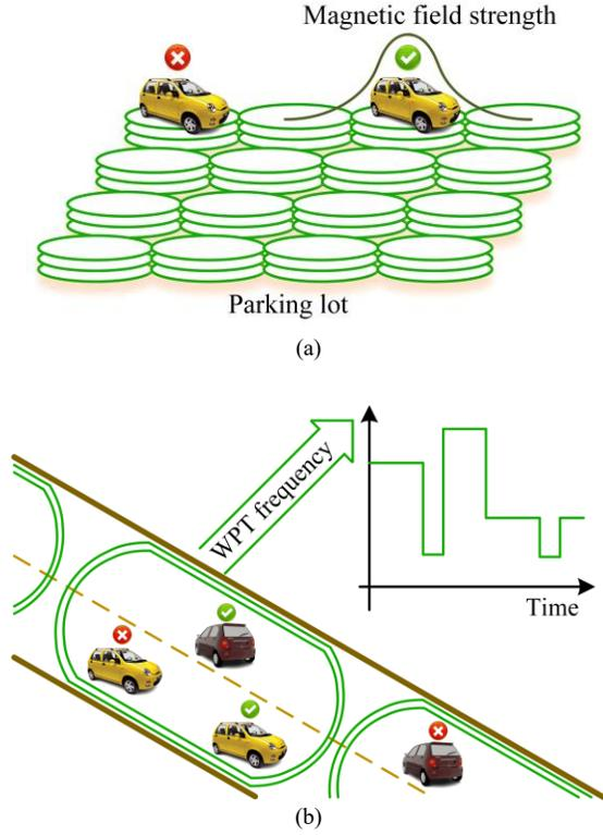
Fig. 1. Current energy protection methods for WPT. (a) Magnetic field editing for static charging. (b) Frequency-variation for dynamic charging.
