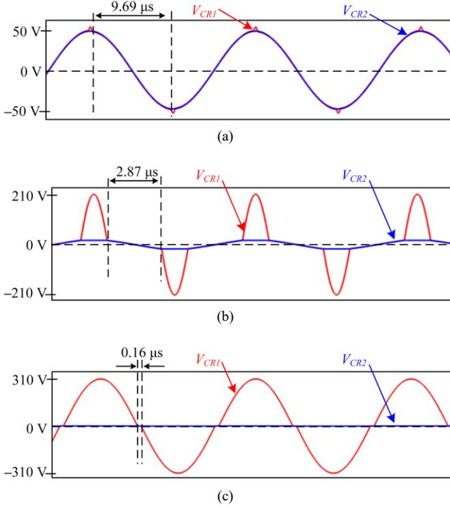
Fig. 11. Voltages of the capacitors for the hacking receiver (a) at 50 kHz, (b) at 120 kHz, and (c) at 300 kHz.
