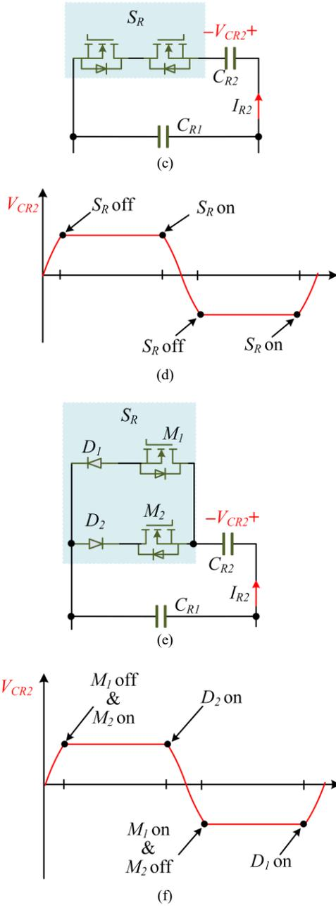
Fig. 9. Various circuits for adaptive capacitor compensation. (a) Single transistor for the capacitor. (b) Asymmetric capacitor voltage. (c) Double transistor as the bidirectional switch for the capacitor. (d) Symmetrical capacitor voltage with four control points. (e) Parallel-transistor-and-diode circuit for switch  $S_R$ . (f) Symmetrical capacitor voltage with two control points.
