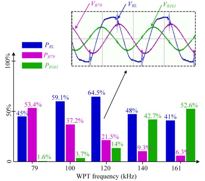
Fig. 17. Percent of energy received by each receiver under different frequencies.
