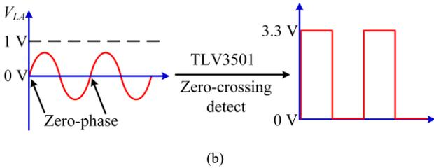
Fig. 8. Frequency and phase detection. (a) Detection circuit. (b) Signal processing.
