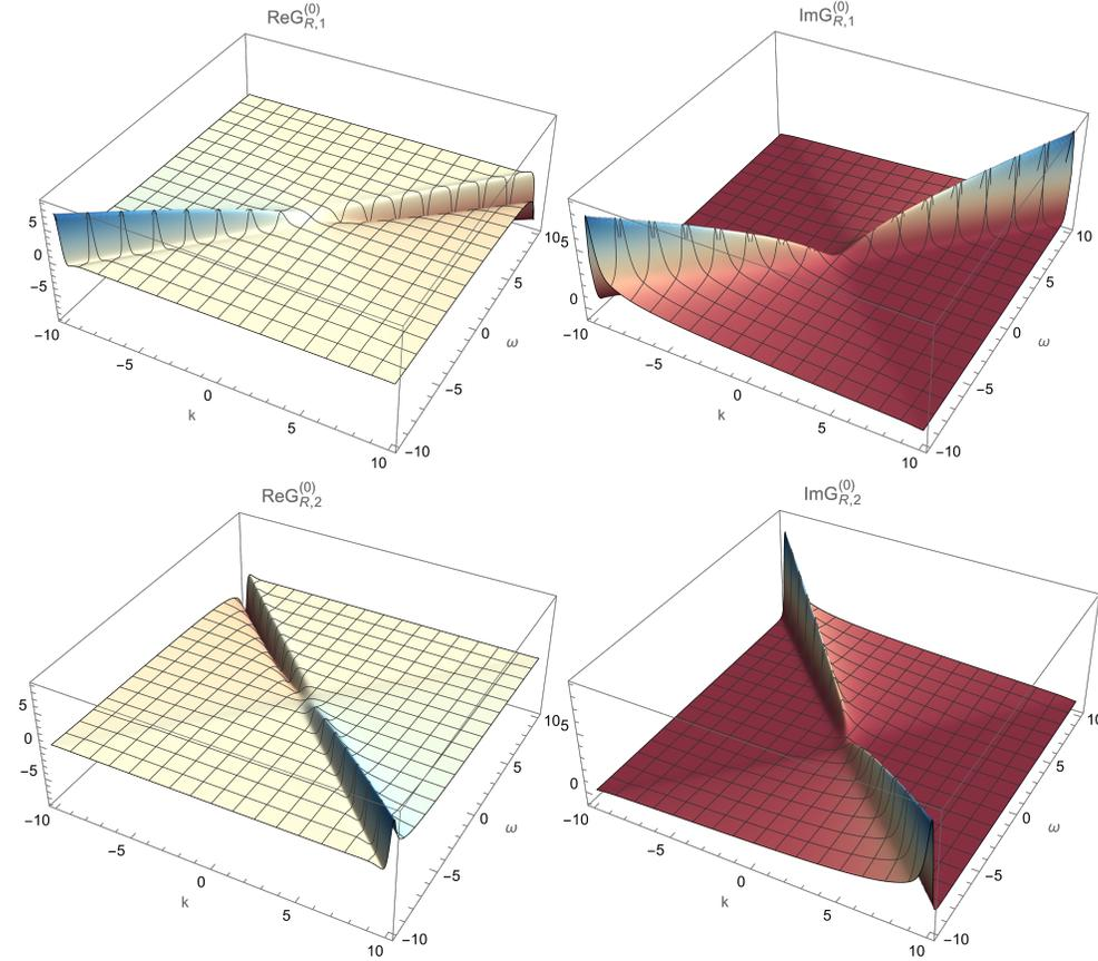
Figure 1: The real and imaginary parts of zero-th order correlation functions  $G_{R,\alpha}^{(0)}$  as functions of  $\omega, k$ . The parameter is chosen as  $q = 0, m = 0.01, z_H = 1$ .
