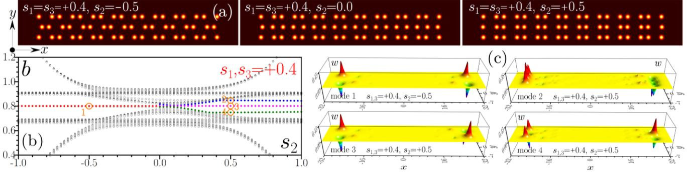
Fig. 2. (a) Examples of three coupled SSH arrays with different shifts of waveguides. (b) Propagation constants of all eigenmodes of the array with  $s_1, s_3 = +0.4$  vs shift  $s_2$  and (c) eigenmodes corresponding to orange circles in (b). Open dots correspond to bulk states, while red, blue, magenta, and olive dots to edge states.
