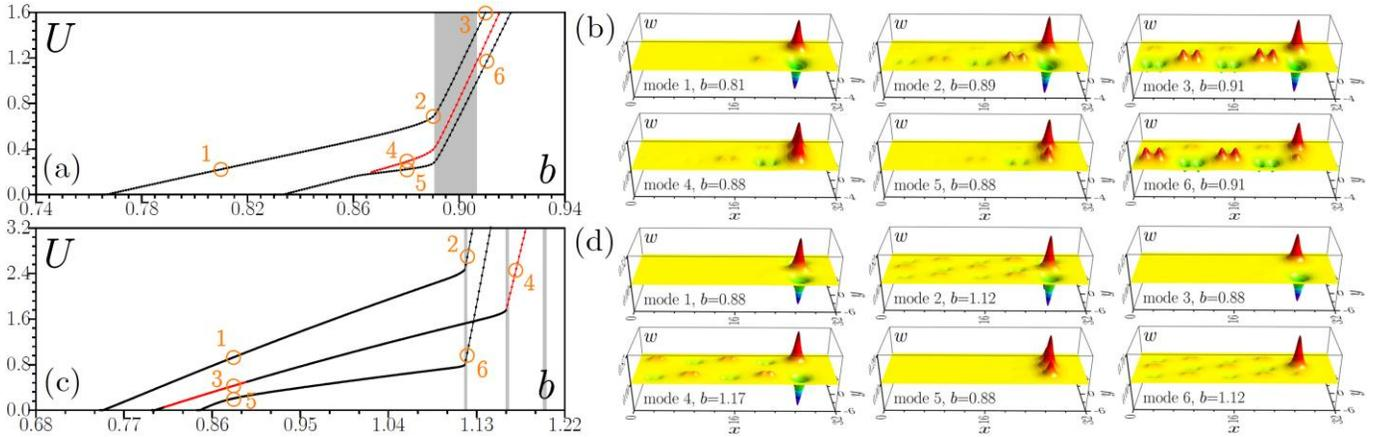
Fig. 3.  $U(b)$  dependencies illustrating families of edge solitons in two coupled SSH arrays with  $s_1 = +0.4, s_2 = +0.8$  (a) and (b) examples of soliton profiles corresponding to the dots in (a).  $U(b)$  dependencies for solitons in three coupled SSH arrays with  $s_1, s_2, s_3 = +0.8$  (c) and (d) examples of their profiles. Grey regions in (a), (c) correspond to the bands of bulk states. Black branches are stable, while red ones are unstable.
