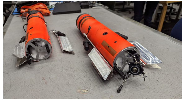
Fig. 6. SpaceSeeds on the workbench right after recovery with the main rotor missing.
