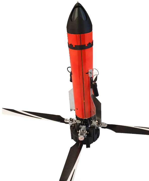
Fig. 2. SpaceSeed with hull, upside-down with respect to falling direction.
