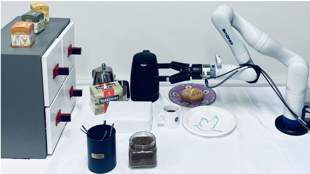
Figure 1: Coffee and plate decoration video. Kinova Gen3 Robot prepares coffee and decorates a plate. Click image for video demonstration.
