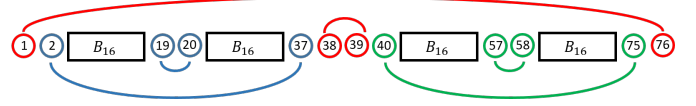
Fig. 1. An example of the recursive construction for z = 4 and t = 19 . We use the companion sets in (9), denoted by B_{16} , as building blocks. Integers within the same companion sets have the same color. The companion sets have cardinality 2.
