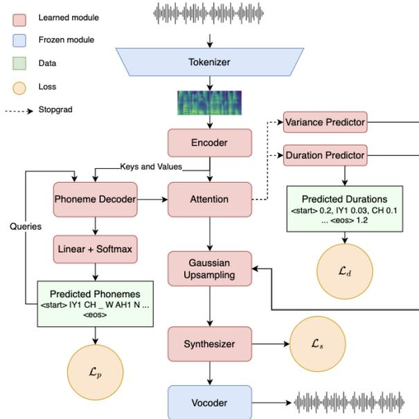
Figure 1: *Architecture Diagram of the proposed DiffuseST Model.*
