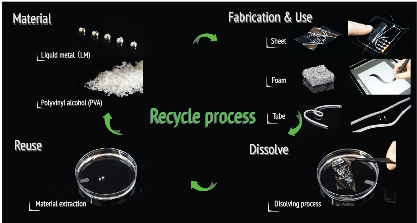
Figure 1: General recycling process for Recy-ctronics. 1: Materials preparation of PVA (substrate material) and liquid metal (electrode material). 2: Different recyclable interactive devices with various form factors (sheet, foam and tube). 3: The dissolving and separation process of the devices. 4: Material extraction for remaking new devices.
