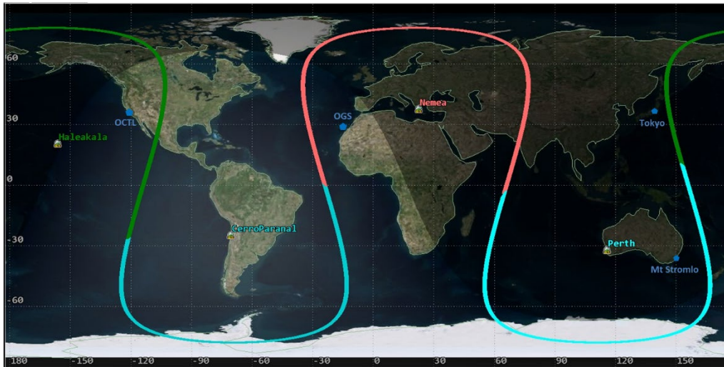
Figure 5. Orbit simulation showing a potential orbit requiring only 4 optical ground stations to support the BHEX science mission. Additional ground stations can be used to improve site diversity.
