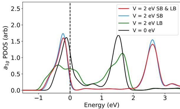
FIG. 4. Vanadium  $a_{1g}$ -orbital PDOS of the M1 phase, obtained by applying an inter-atomic potential of  $V = 2$  eV to both SB and LB (red line) or to either SB (cyan line) or LB (magenta line) vanadium-vanadium pairs. The black line shows the case with  $V = 0$  eV. Fermi level at 0 eV shown by the dashed line.
