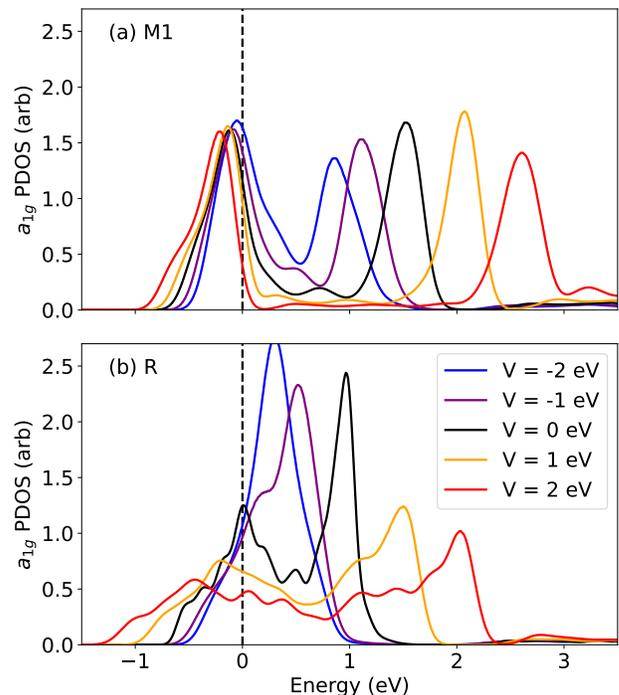
FIG. 3. Vanadium  $a_{1g}$ -orbital PDOS for different positive and negative values of  $V$  (shown in red and blue color gradient respectively, with  $V = 0$  in black) applied on both bonds for (a) M1 and (b) R structures of  $\text{VO}_2$ . Fermi level at 0 eV shown by the dashed line.
