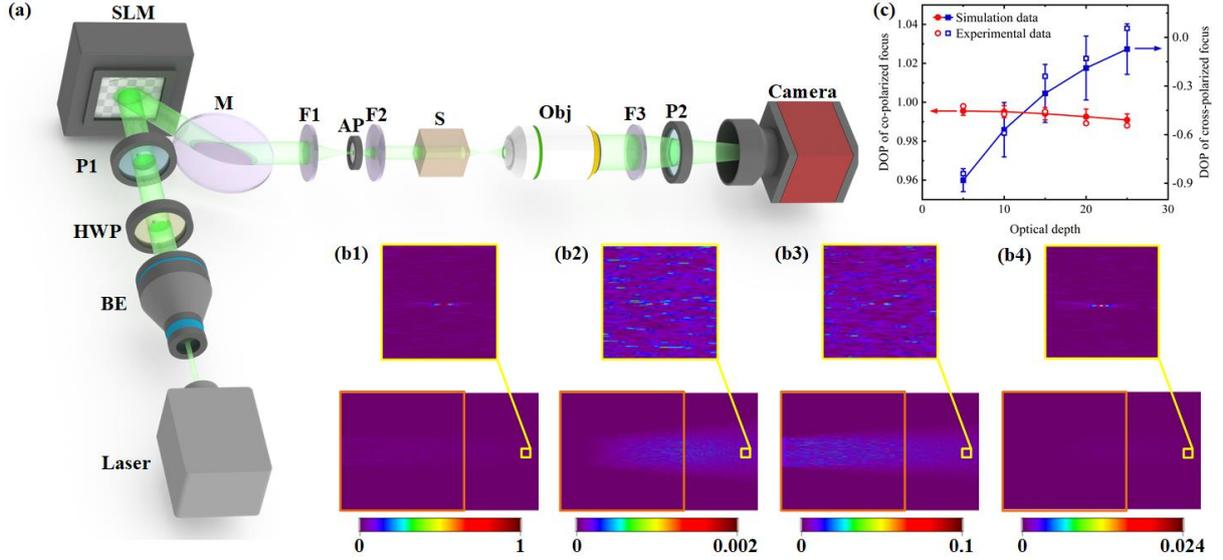
**Figure 4.** Focusing of vector light through the scattering medium. a) Experimental setup, BE: beam expander, HWP: half-wave plate, P1, P2: polarizer, SLM: spatial light modulator, M: mirror, F1, F2, F3: lens, AP: aperture, S: scattering medium, Obj: objective; b1-b2) focus formed with  $T_x$ ; b3-b4) focus formed with  $T_y$ ; c) DOP of co-polarized and cross-polarized focus.
