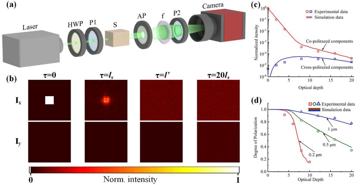
**Figure 3.** Light transmission in turbid medium. a) Experimental setup, HWP: half-wave plate, P1, P2: polarizer, S: scattering medium, AP: aperture, f: tube lens; b) evolution of the light field distribution with increasing penetration depth; (c) intensity transmission as a function of the optical depth; d) degree of polarization as a function of the optical depth with different diameters of the particles (0.2 $\mu\text{m}$ , 0.5 $\mu\text{m}$ , 1 $\mu\text{m}$ ).
