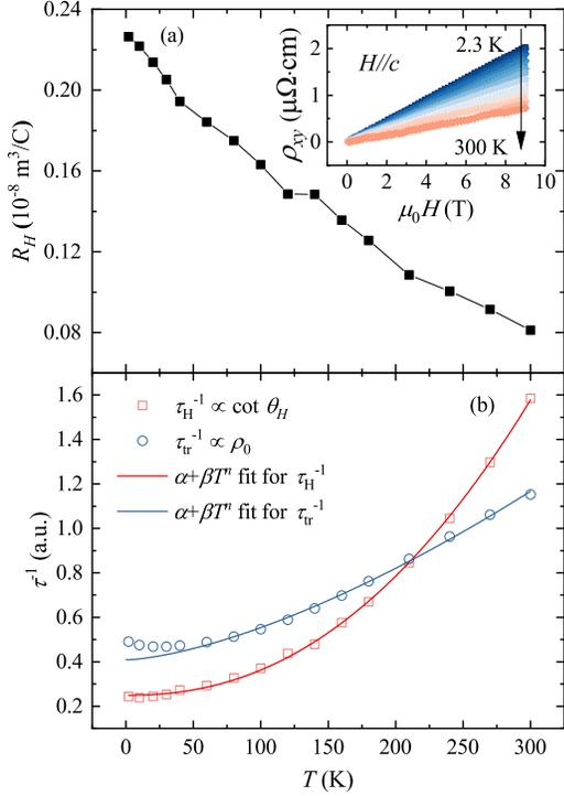
Figure 4. (a) Temperature dependence of the Hall coefficient  $R_H$  for sample SH3. The inset shows the magnetic field dependence of  $\rho_{xy}$  at different temperatures. (b) Temperature dependence of  $\tau_H^{-1}$  and  $\tau_{tr}^{-1}$ . The solid lines show the fit by  $\alpha + \beta T^n$  with  $n = 2.24 \pm 0.03$  for  $\tau_H^{-1}$  and  $n = 1.50 \pm 0.08$  for  $\tau_{tr}^{-1}$ .
