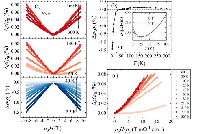
Figure 5. (a) Field dependence of MR  $\Delta\rho/\rho_0$  for sample SH3 at different temperatures. (b) Temperature dependence of the magnetoresistance at 9 T. The inset shows the  $\rho - T$  curve at 0 T and 9 T. (c) The positive MR plotted by following Kohler's law at different temperatures.
