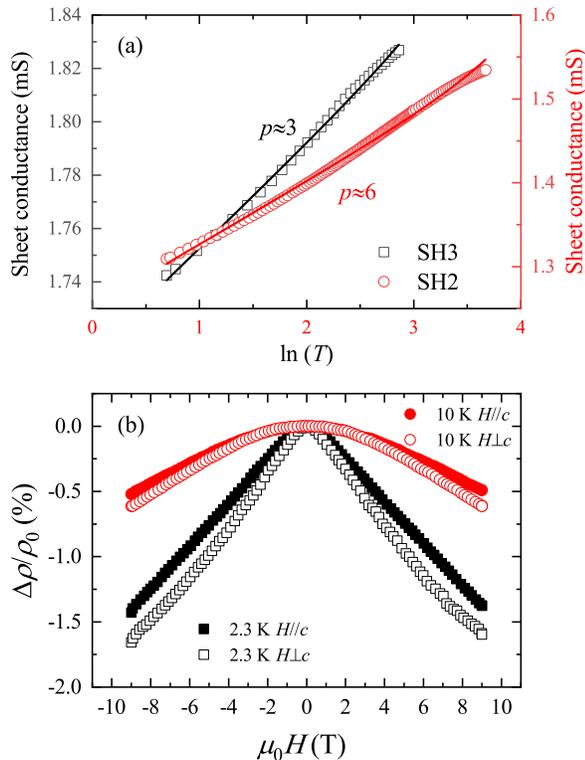
Figure 8. (a)  $\rho-T$  curves and fits to the model of weak localization (eq. 4) at low temperatures for two metallic samples. (b) Magnetoresistance in the magnetic field applied parallel and perpendicular to the  $\text{La}_3\text{Ni}_2\text{O}_{7-\delta}$  film  $c$ -axis for sample SH3.
