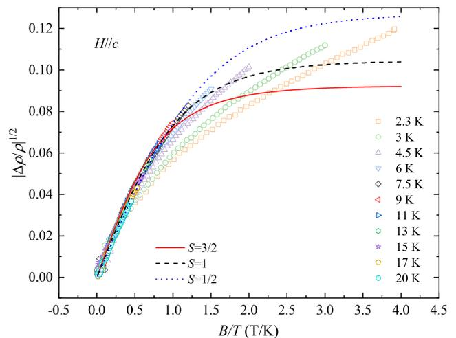
Figure 7. The square root of  $|\Delta\rho/\rho_0|$  versus  $B/T$  at low temperatures. The solid, dashed and dotted lines in red, black, and blue represent the Brillouin function fits (eq. 3) for  $T \geq 7.5$  K with  $S = 3/2, 1,$  and  $1/2$ , respectively.
