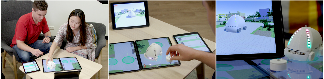
Figure 1: We present a tangible multi-display toolkit to inform the design of AV-pedestrian interfaces. The toolkit contains a) computer simulations across multiple displays to capture different viewing angles, b) tangible objects to interact with the simulated environment and to simulate the interface’s behaviour through an integrated LED display, and c) a configuration app allowing participants to change the interface’s behaviour in real-time.
