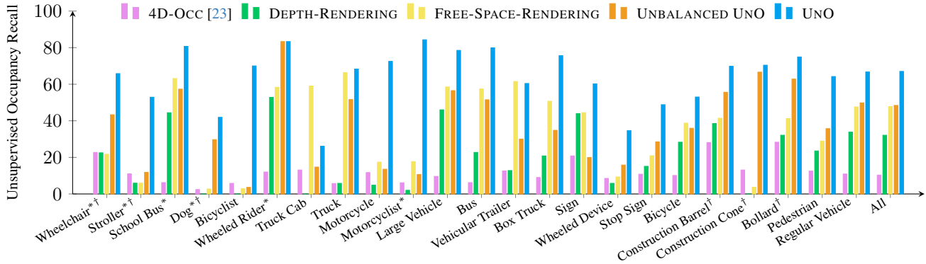
Figure 7. Unsupervised occupancy recall comparison on the Argoverse 2 Sensor dataset, averaged across the prediction horizon. Recall is computed at a precision of 0.7. * denotes the rarest 25% of classes, and † denotes the smallest (by bounding box volume) 25% of classes.
