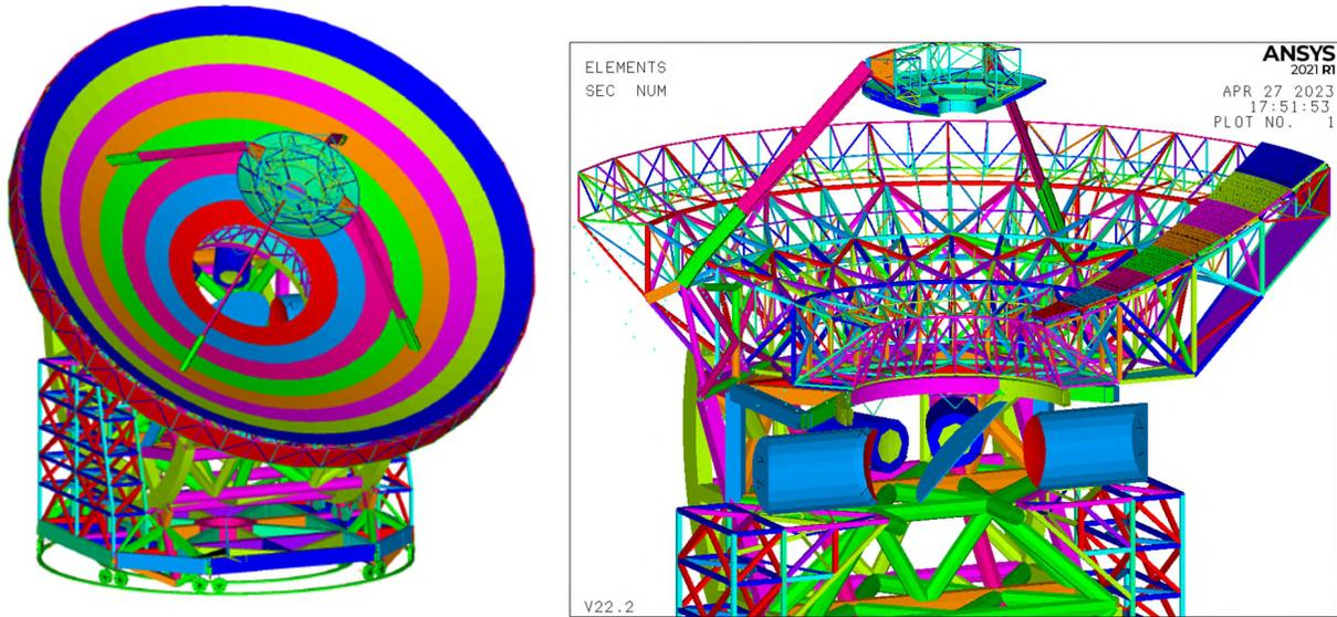
Figure 6: Finite element model of the full telescope. Left: full model view. Right: cut view along the elevation axis
