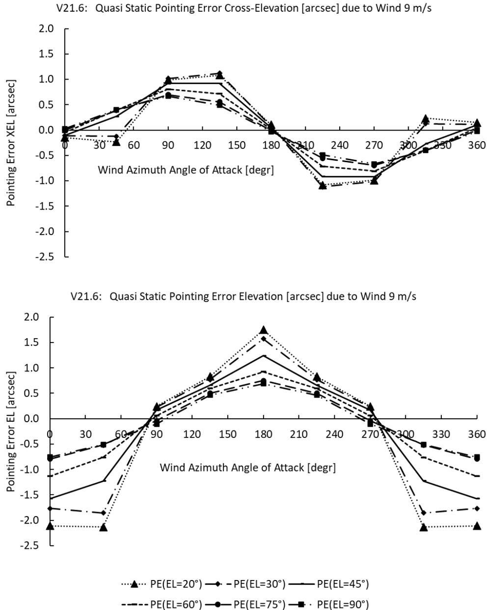
Figure 13: Upper: Pointing Error in Cross-Elevation Direction (perpendicular to momentary elevation direction). Lower: Pointing error in EL due to continuous, quasi-static wind-load 9 m/s (one line per elevation position).
