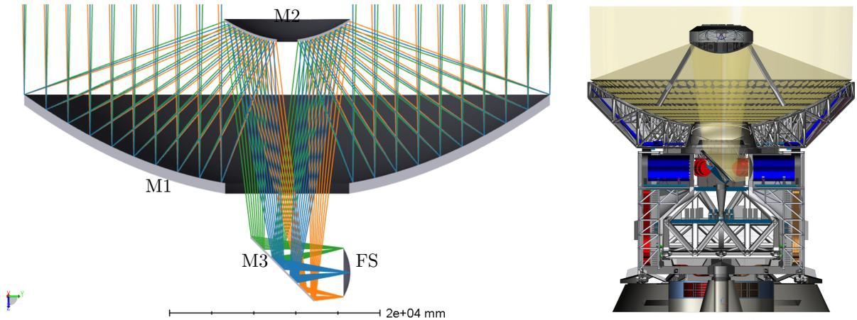
Figure 1: Left: The optical layout for AtLAST, reproduced from Mroczkowski et al. 2024.<sup>2</sup> The primary, secondary, and tertiary mirrors (M1, M2 and M3, respectively) concentrate and direct light from the sky onto the focal surface (labeled “FS”). Right: A rendering of the AtLAST CAD model including the optical path in gold. The CAD model, shown in Figures 3 & 4, is described in more detail in this section as well as Mroczkowski et al. 2024.<sup>2</sup>
