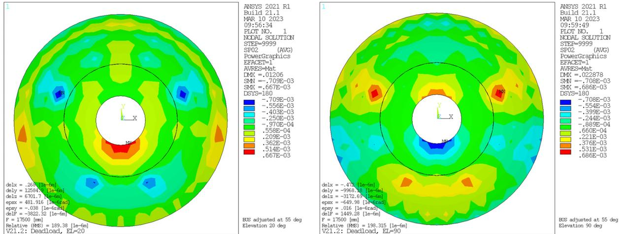
Figure 7: M1 surface deformation under gravity at elevation positions of 20° and 90°, demonstrating the compliance with the requirement of < 200 μm rms (before active corrections).
