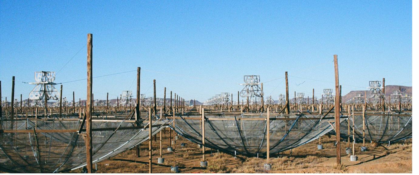
**Figure 1.** Photo of the Phase II HERA antennas. This view highlights the fact that many pairs of feeds have unobstructed views of each other and motivates the feed-to-feed re-radiation model of mutual coupling presented in Section 2.
