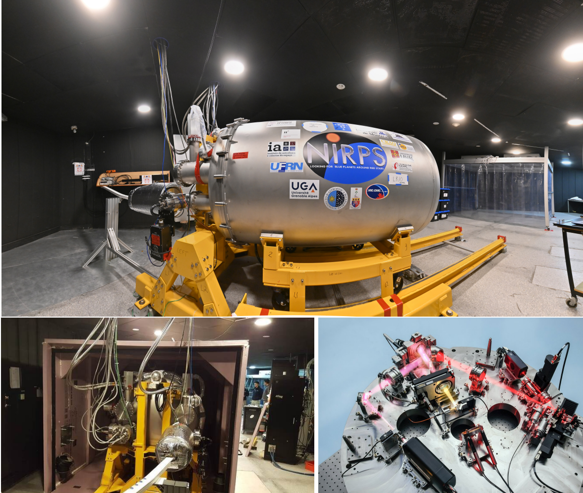
Figure 1. [Top] Wide-angle view of the NIRPS back end prior to the addition of the thermal enclosure. Fibres arrive from the left the the cryostat. [Bottom left] Back end in the thermal enclosure prior closing it. The cylinder enclosed in aluminized wrapping contains the double-scrambler. [Botton right] Lab view of the NIRPS front-end with the optical path highlighted.
