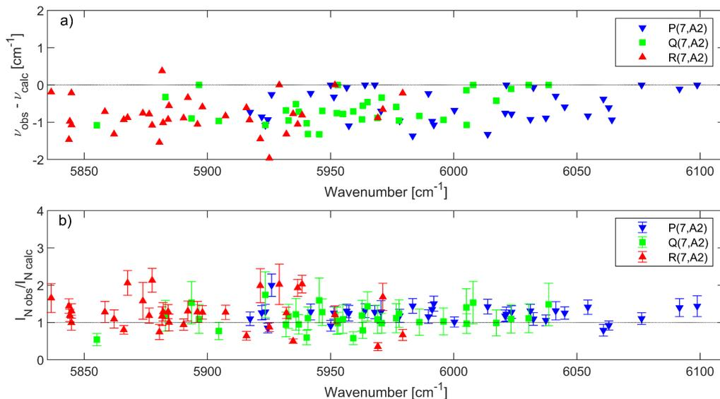
Figure 10. a) The difference between the observed center wavenumbers and those predicted by ExoMol for ladder-type OODR lines detected in the measurements with three different pump transitions, as marked in the legend. b) The ratios of the normalized intensities obtained from the three measurements to those calculated based on data from the ExoMol and HITRAN. The error bars show  $1\sigma$  uncertainties, and they are negligibly small in a).
