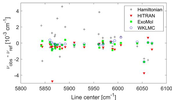
Figure 11. A comparison of the observed center wavenumbers of the V-type features to the effective Hamiltonian (black crosses), HITRAN (red triangles), ExoMol (green squares), and WKLMC line list (blue circles). The experimental uncertainties are negligible compared to the scatter.
