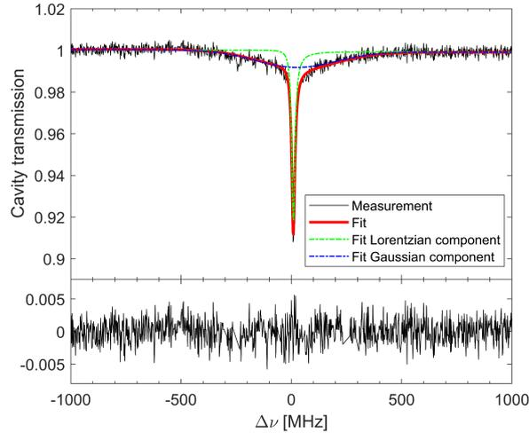
Figure 4. The sub-Doppler ladder-type OODR transition at  $5956.54279(1)$   $\text{cm}^{-1}$  in the  $P(7, A_2)$ -pumped spectrum (black) and the fit (red solid curve) plotted as a function of the detuning,  $\Delta\nu$ , from the center of the transition. The dashed curves show the Gaussian (blue) and Lorentzian (green) components of the fit respectively, and the bottom panel shows the residuals.
