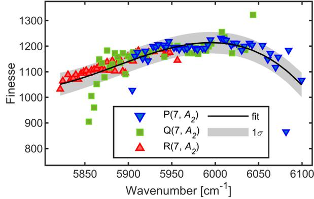
Figure 3. The cavity finesse retrieved from fits to the Doppler-broadened lines in the three interleaved and baseline-corrected background spectra, with pump on the  $P(7, A_2)$ ,  $Q(7, A_2)$  and  $R(7, A_2)$  transition (downward blue triangles, green squares, upward red triangles, respectively), together with a polynomial fit (black curve) and  $1\sigma$  confidence interval (shaded region). The error bars on the individual finesse values are negligible on this scale.
