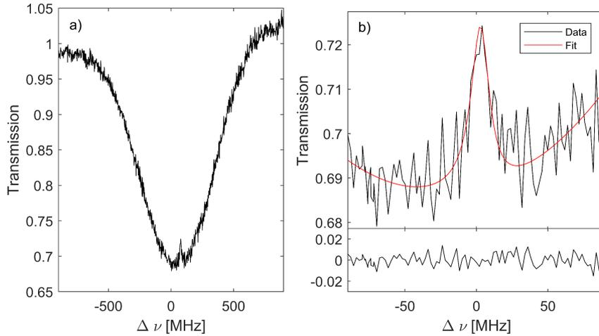
Figure 5. a) The  $2\nu_3 Q(7, A_2)$  line with the V-type transition in the  $Q(7, A_2)$ -pumped spectrum. b) A zoom-in on the V-type transition (black) and the corresponding fit (red). Residuals are shown in the bottom panel.
