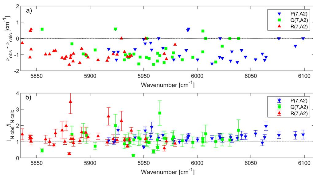
Figure 9. a) The difference between the observed center wavenumbers and those predicted by TheoReTS/HITEMP for ladder-type OODR lines detected in the measurements with three different pump transitions, as marked in the legend. b) The ratios of the normalized intensities obtained from the three measurements to those calculated based on data from the TheoReTS/HITEMP and HITRAN. The error bars show  $1\sigma$  uncertainties, and they are negligibly small in a).
