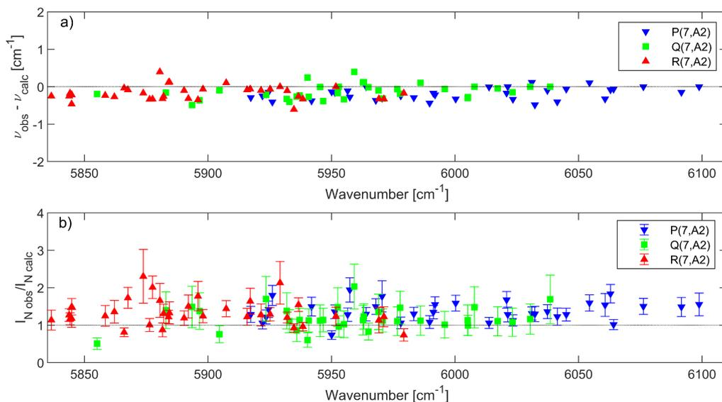
Figure 8. a) The difference between the observed center wavenumbers and those predicted by the effective Hamiltonian for ladder-type OODR lines detected in the measurements with three different pump transitions, as marked in the legend. b) The ratios of the normalized intensities obtained from the three measurements to those calculated based on data from the Hamiltonian and HITRAN. The error bars show  $1\sigma$  uncertainties, and they are negligibly small in a).
