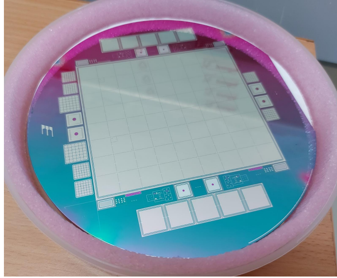
Figure 4: Photograph of fabricated Si pad array on a 6-inch n-type Si wafer.
