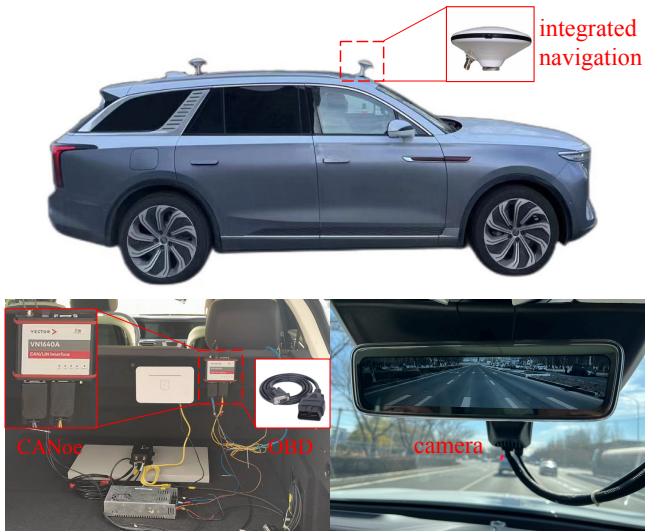
Fig. 1: Architecture of data-acquisition system
