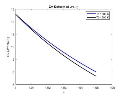
Figure 3.  $C_V$ .vs.  $\eta$  at different temperatures (K).
