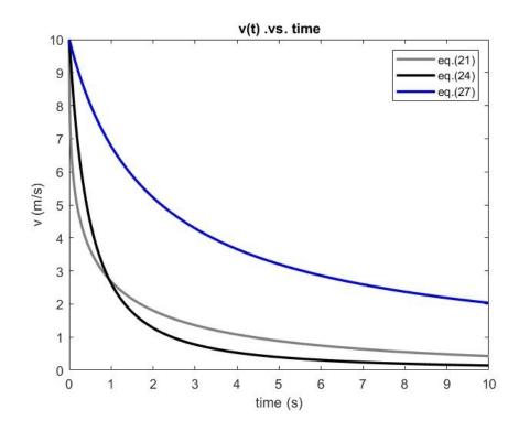
Figure 1. Simulations for the solutions of Langevin equation, eqs. (21, 24 and 27). The parameters used were  $v_0=10\text{m/s}$ ;  $\lambda=0.5$ ;  $\alpha=0.38$ ;
